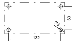
Drilling plan for mounting plate
